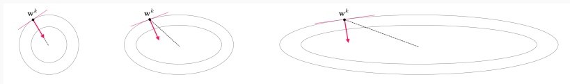
Figure 3: Sequential illustrations from left to right show that in more elongated contours of a two-dimensional quadratic, the gradient descent direction (in red) increasingly diverges from the optimal path (dashed black) that connects w^k to the minimum at the center.
